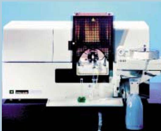
Figure 7 Flame emission spectrophotometer (photograph by courtesy of Pekin Elmer Ltd)
